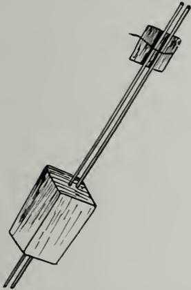
Shows section of double-tube rod used as a guide for fixing position of wires to backing for soldering.
