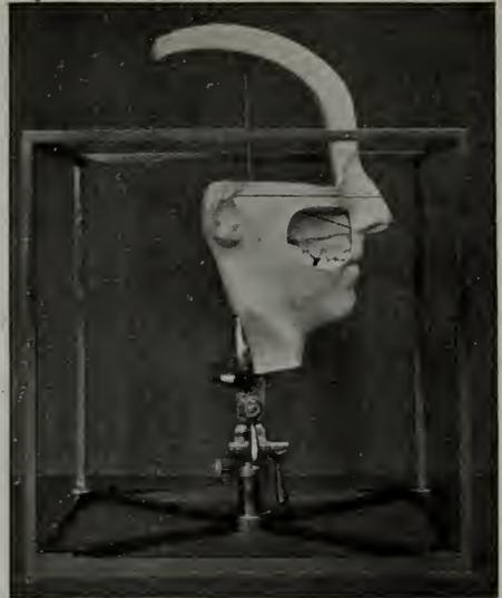
FIG. 6: *Cubus craniophor*, with plaster facial cast and model in the right position, adjusted according to the Frankfort horizontal line. Both tragia are brought to the same height by moving the head in the second joint.
