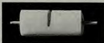
Cut made in porcelain rod No. 25 with a brass wheel, using Columbia lathe at lowest speed with carborundum powder and sugar mixture. Time taken, 70 sec.
