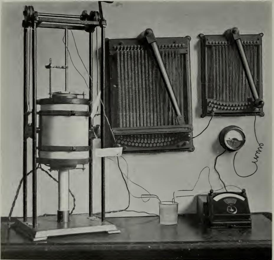
peratures obtained is marked off on the vertical axis (see Fig. 4), and the time on the horizontal axis. The intersection of these co-ordinates gives us a succession of points, which in the case of "10" will give us the lines shown, from which the fusing-point, in this case  $226^{\circ}\text{C}.$ , may be read off immediately. (For metals with a higher fusing-point the
