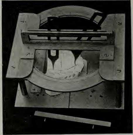
FIG. 18: Symmetroscope—the model being placed with the median line on the short arm of the cross on the basal plane. The bridge is pushed forward, the two tracing-tools indicating the distance from the first bicuspid to the raphe.
