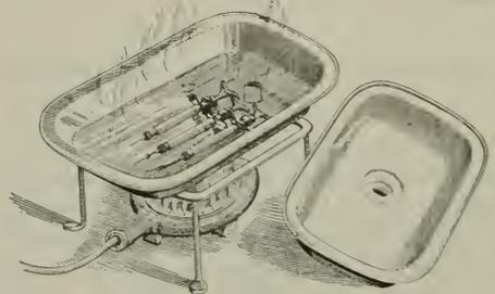
etc.; also an iron stand and a suitable gas burner for heating (see figure).
